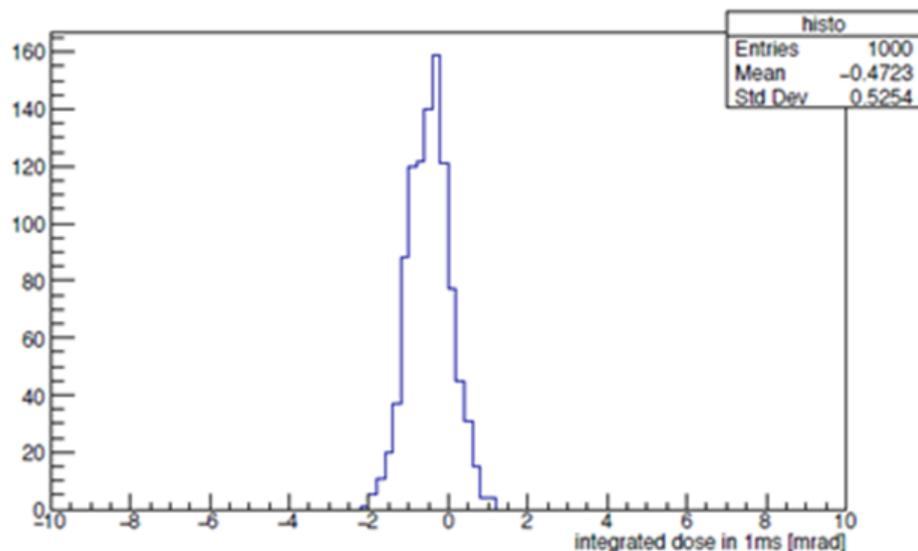
Figure 3.13: Dose-rate distribution of 100 kHz pedestal data summed in independent 1-ms-time intervals; the standard deviation is of  $\approx 0.5$  mrad, much lower than the "fast" threshold set.
