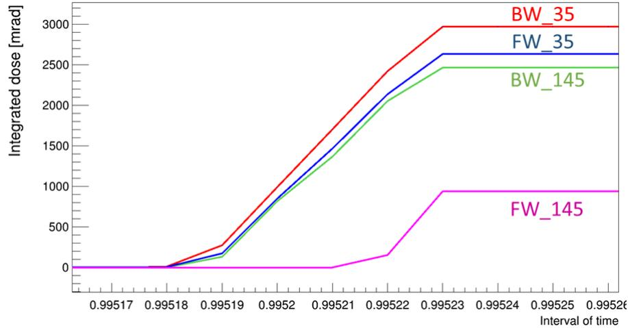
Figure 3.16: Integrated dose as a function of time for the four abort diamonds (DCU 1). The integration is performed in a moving 1 ms-window, updated every 10  $\mu$ s. The integrals reach their maxima when the beams are actually aborted and the beam losses go to zero
