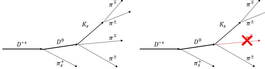
Figure 4.3: Conceptual sketch of (left) a fully and (right) a partially reconstructed  $D^{*+} \rightarrow D^0[\rightarrow K_S^0(\rightarrow \pi^+\pi^-)\pi^+\pi^-]\pi^+$ , decay. The probe track is a pion from the  $D^0$  decay while the  $K_S^0$  pions are always reconstructed.
