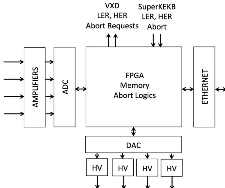
Figure 3.3: Block diagram representing the main DCU functional components.
