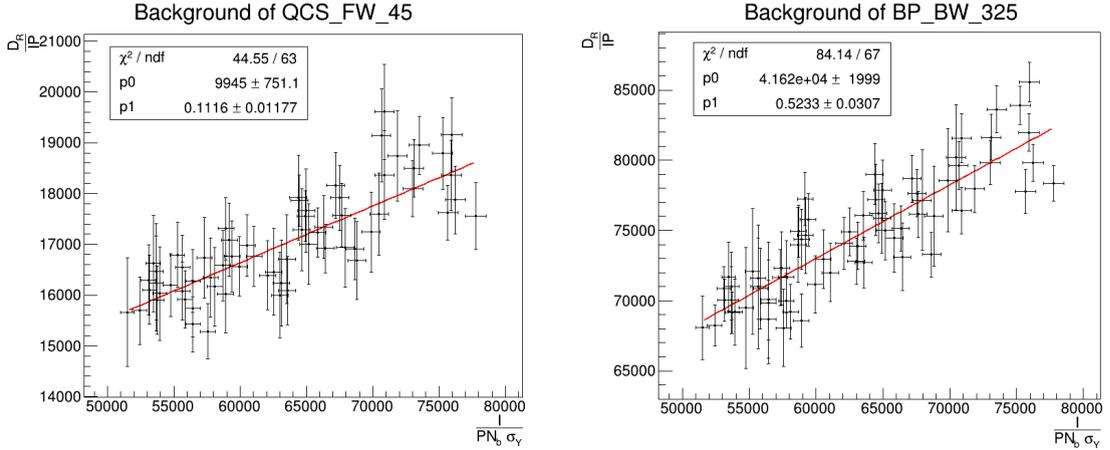
Figure 3.18: Results of the fit of dose-rate data seen by two diamonds.
