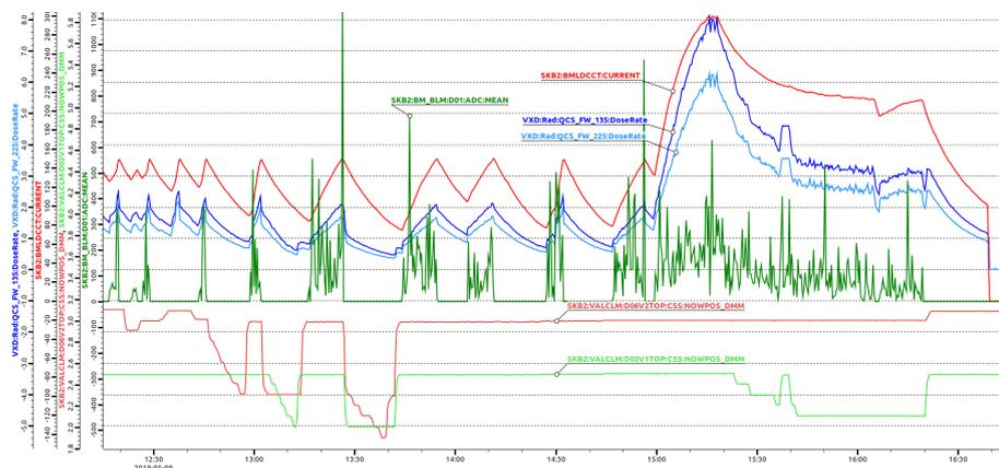
Figure 3.6: Diamonds dose rates (blue and light-blue), LER beam current (red), collimators aperture (orange and light-green), and SuperKEKB loss monitor (green) archived data, displayed as a function of time. I used such plots to explore correlations between different variables.
