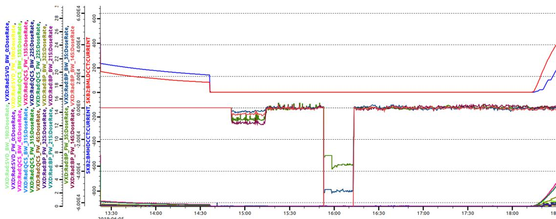
Figure 3.7: Beam currents (red and blue lines) and diamond dose rates (other colored lines) as functions of time. Various shifts of pedestal values were observed while beams were off and I was working on the DCUs configuration.
