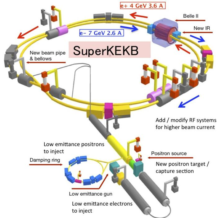
Figure 2.3: Scheme of the SuperKEKB collider.
