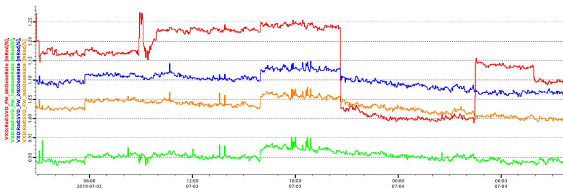
Figure 3.11: DCU 4 diamonds dose rates as a function of time (one color per sensor). The anomalous behavior of the SVD\_FW\_60 signal (red line) is evident, with spikes and several pedestals shifts with no such changes in the other diamonds.
