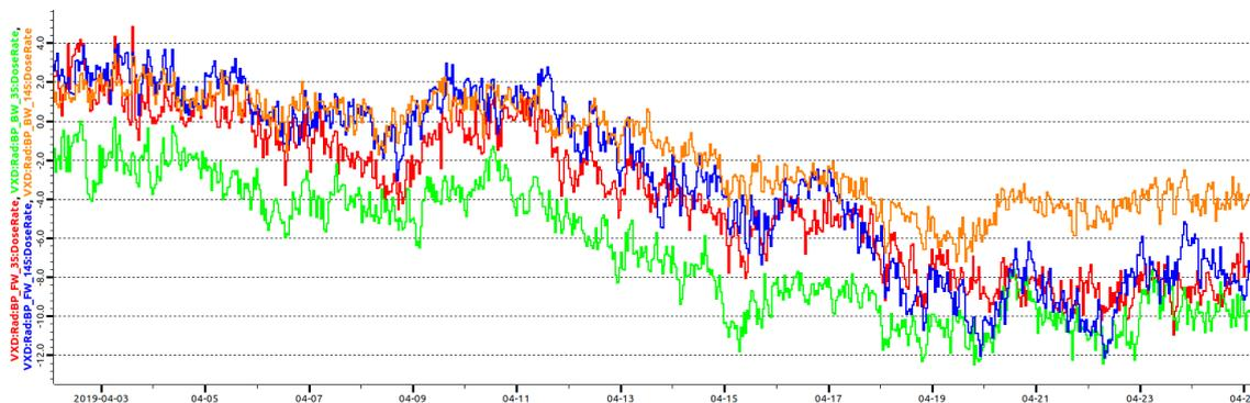
Figure 3.8: Beam-pipe diamonds (one color per sensor) dose rates as functions of time during a long period without circulating beams (April 3rd to April 25th). Pedestal drifts of more than 10 mrad are evident.
