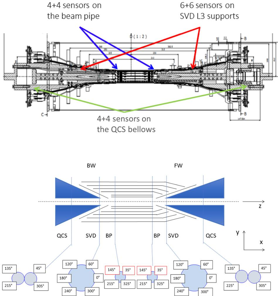
Figure 3.2: Radiation-monitor diamond sensors in the Belle II Phase 3 setup. Eight sensors are installed on the beam pipe, twelve on the SVD support, and eight on the QCS magnets bellows. Azimuthal position and labelling of each diamond is shown. Only the four diamonds indicated with red boxes in the bottom panel are used to deliver the beam-abort signal, the others monitor radiation.
