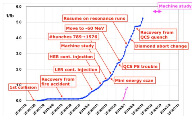
Figure 2.4: Plot summarizing the main events that characterized SuperKEKB operations in the 2019 spring run.
