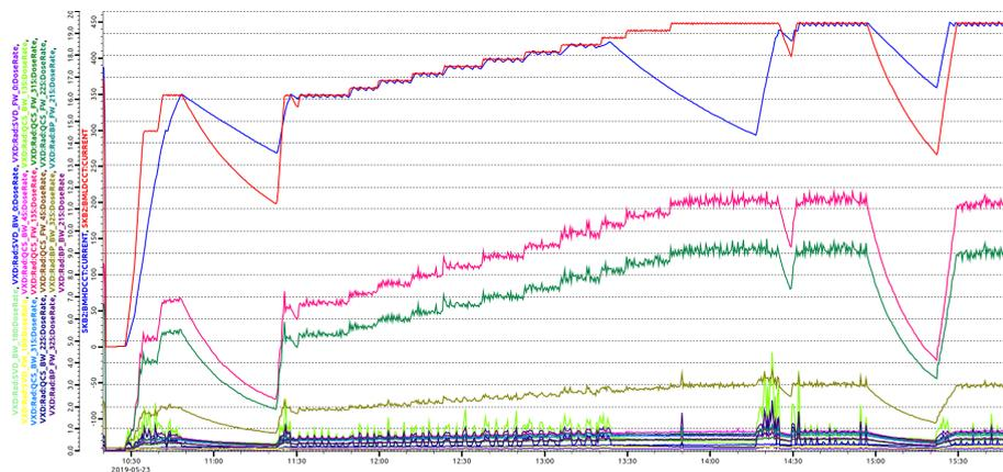
Figure 3.5: Screenshot of a live plot of beam currents (red and blue lines) and diamond readouts (other colored lines) as a function of time. I used this live plot to observe diamond behaviour when currents were being increased.
