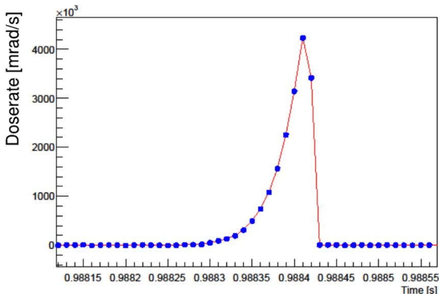
Figure 3.14: Dose-rate seen by BP\_FW\_45, as a function of time, in the QCS quench of June 6th, 2019. With the new dynamic range, the diamond signal did not saturate and the full background radiation spike is properly sampled.
