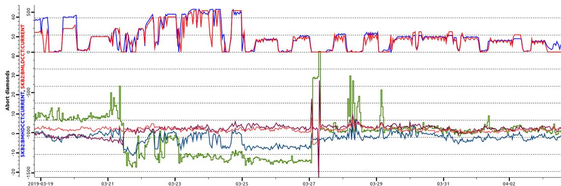
Figure 3.10: Beam currents (red and blue lines) and DCU 1 diamond dose-rates (other colored lines) as a function of time during early Phase 3.
