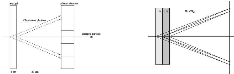
Figure 2.10: Scheme of the ARICH detector.
