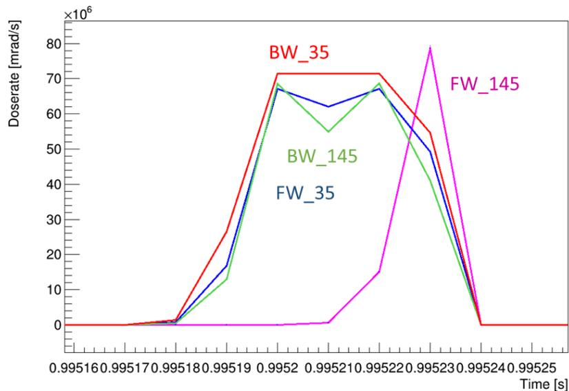
Figure 3.15: Dose rate as a function of time for the four abort-enabled diamonds (DCU 1).
