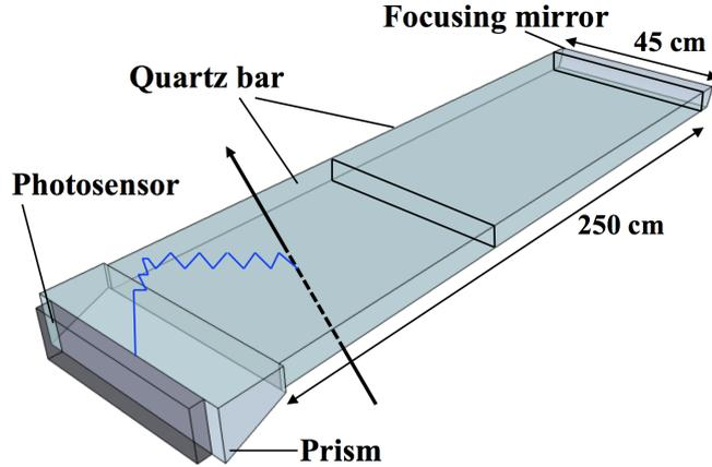
Figure 2.9: Scheme of a TOP bar. A charged particle crossing the radiator and emitting Cherenkov photons, which are collected at the PMT, is also represented.
