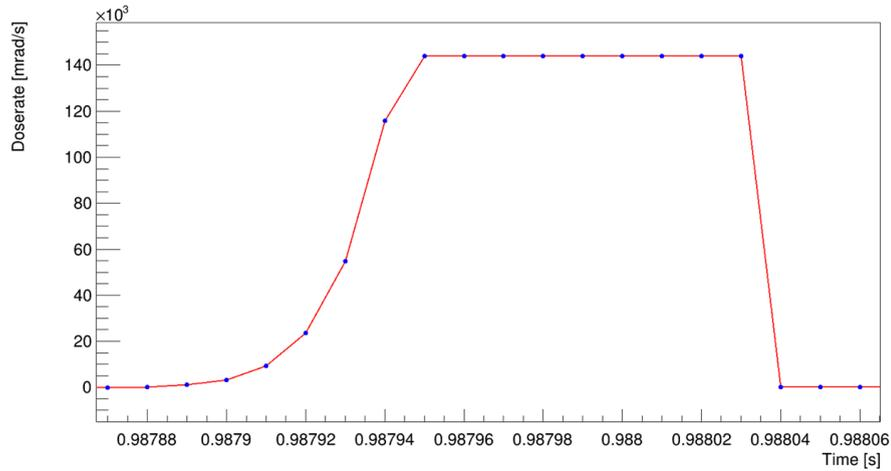
Figure 3.12: Dose rate seen by the most affected diamond as a function of time, for the QCS quench event of May 28th. The clipping at  $\approx 146$  mrad shows that the high dose saturated the readout.
