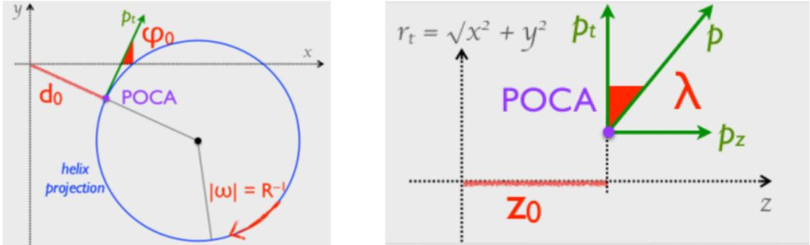
Figure 4.2: Illustration of the helix parameters used in track parametrization at Belle II. The parameter  $\omega$  is not shown.
