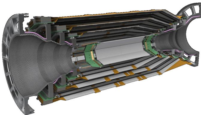
Figure 2.7: Exploded view of a SVD detector half.
