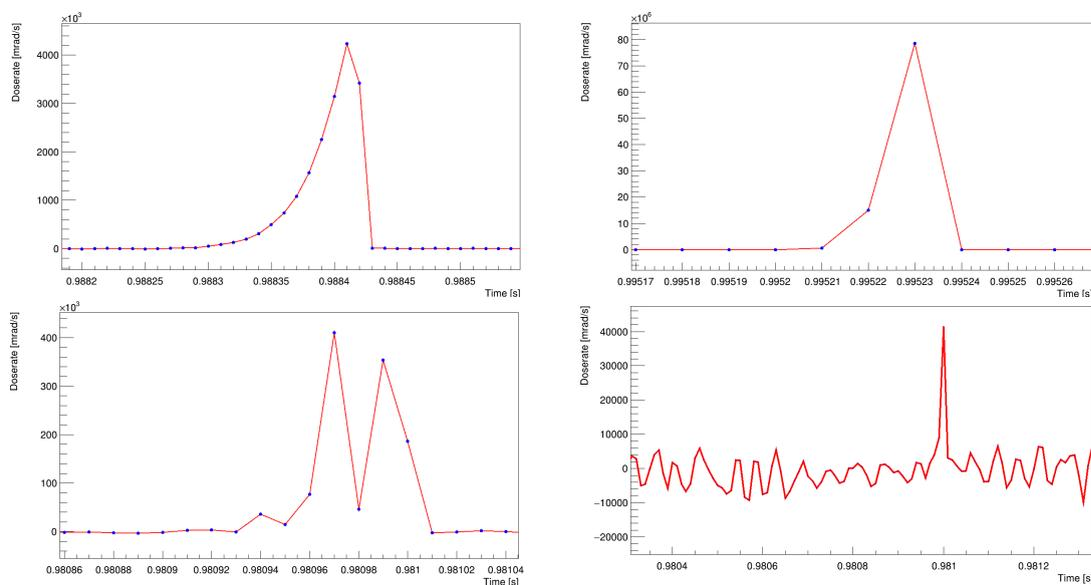
Figure 3.9: Examples of dose rate seen by diamonds in various aborts as a function of time. The top panels show dose-rate associated with losses that triggered diamond aborts. The bottom left plot shows a peculiar dose-rate shape. The bottom right plot shows the dose-rate corresponding to an abort issued by another SuperKEKB loss monitor: a background spike is visible, but the dose-rate seen by diamonds is lower in this case with respect to the three other examples.
