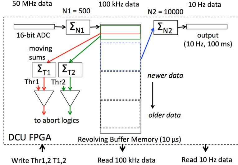
Figure 3.4: Block diagram representing the DCU data stream.
