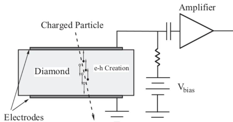
Figure 3.1: Schematic layout of a diamond sensor.
