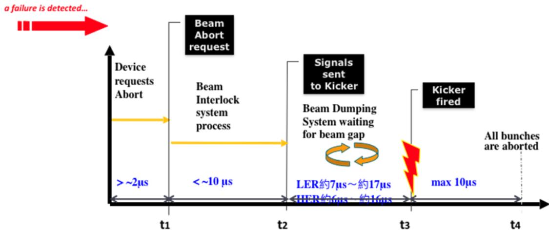
Figure 3.17: Scheme of the abort delays: the contributions to the total delay are shown.
