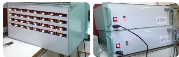
Figure 1: (Left) 32-axis controllers. (Right) Two 32-axis controllers looped together.
