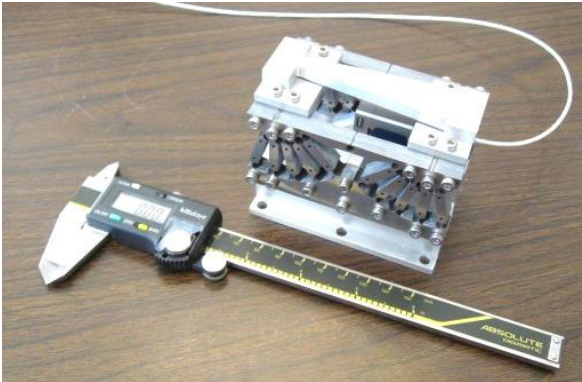
Figure 10: Photograph of the Z7-5006 prototype dynamic mirror bender with closed-loop control configuration.
