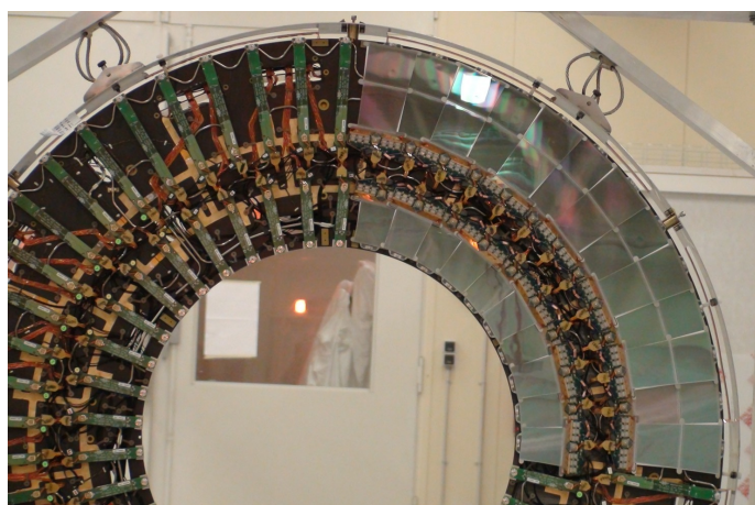
Figure A.2: The 33 end cap modules, (13 outer, 10 middle and 10 inner) attached to the disk quadrant.
