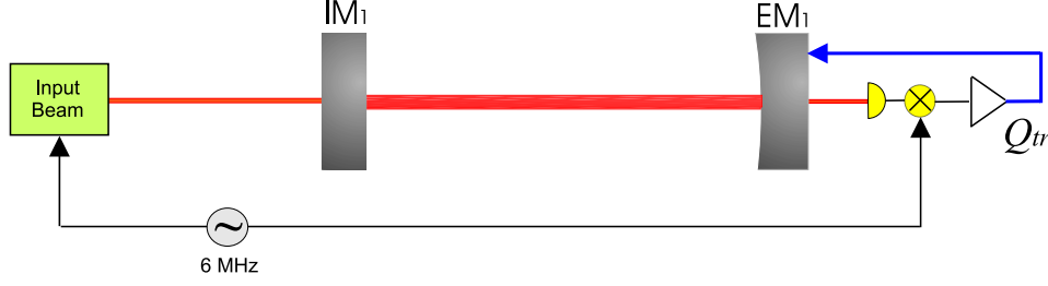
Figure 3.5: Locking scheme of the single Fabry-Perot cavity. The Pound-Drever-Hall signal extracted in transmission to the cavity is filtered in order to derive a controller proportional to the relative velocity of the mirrors, and is fed back to the end mirror.
