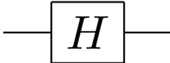
Figure 2. Pictorial representation of Hadamard gate in a circuit.
