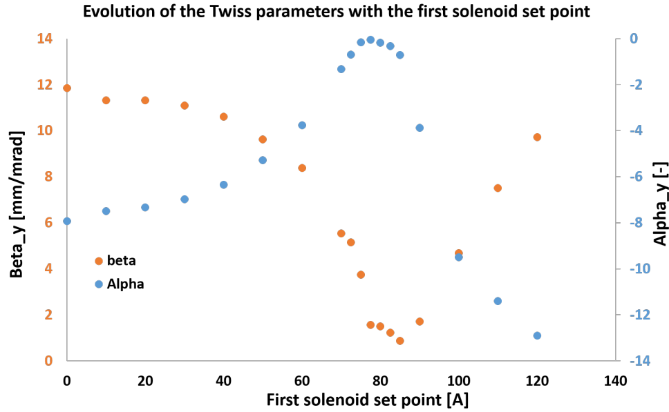
Figure 3.14: Evolution of \alpha_y and \beta_y in the middle of the LEBT with respect to the first solenoid setpoint I_1^{sol} .
