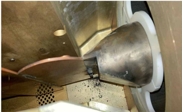
Figure 3: Damage by arcs to forward input port of a circulator.
