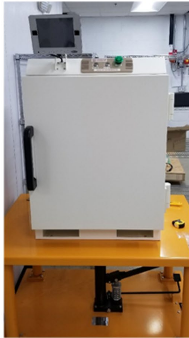
Figure 5: Ludlum Model S4A SAM installed at STERIS Libertyville X-ray RTC center
