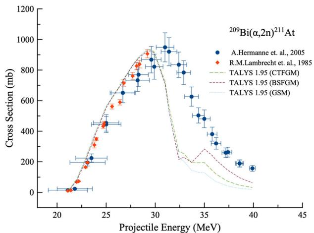
**Fig. 3** Experimental data against the recommended fit for  $^{209}\text{Bi}(\alpha,2n)^{211}\text{At}$  reaction
