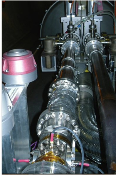
Figure 2: A photograph of one of the two ATLAS BPTX stations.
