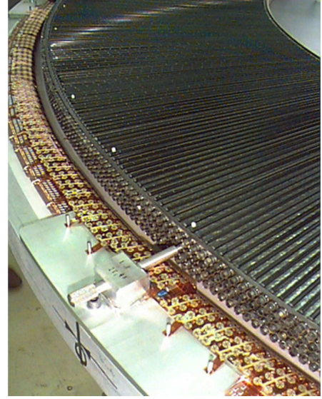
Figure 20: Photograph of a four-plane TRT end-cap wheel during assembly. From Ref. [27].
