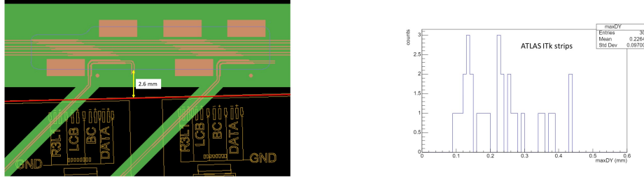
Figure 6. Detail of CAD layout for a barrel bus tape showing edge of silicon module (red), at high voltage and exposed bond pads at low voltage (left). The minimum nominal separation between an exposed bond pad and the edge of the sensor in this area is 2.6 mm. Measured distortion (see text for explanation) for production barrel bus tapes after co-cure (right).
