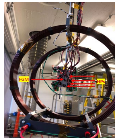
Figure 1: Hall probes calibration setup.
