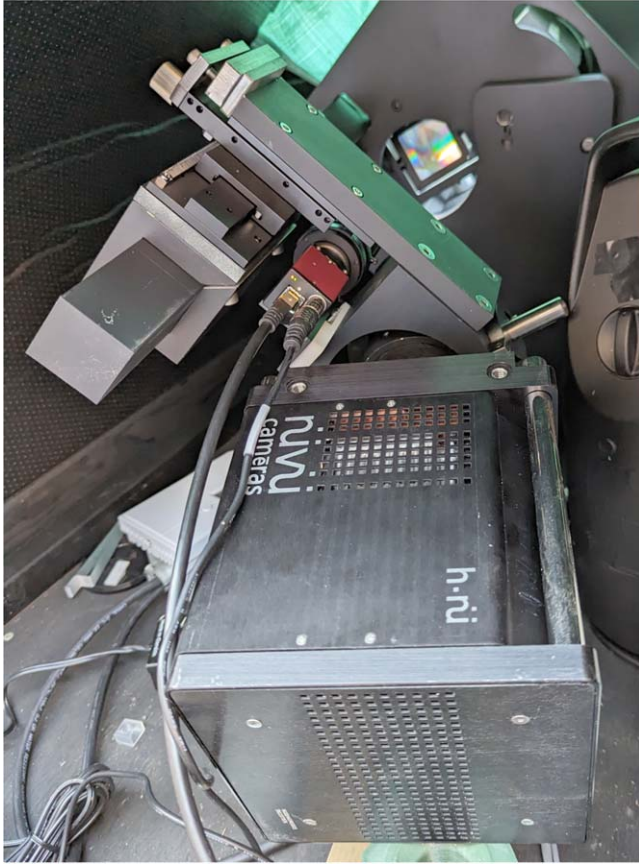
Figure 2. The CAMO-S system showing the EMCCD spectral camera (bottom) and direct camera (red camera at top). The grating can be seen at the top center through the opening in the galvanometer mount.
