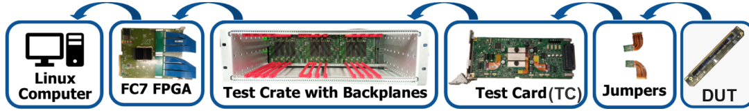
Figure 2. Simplified diagram of the crate-based test system.
