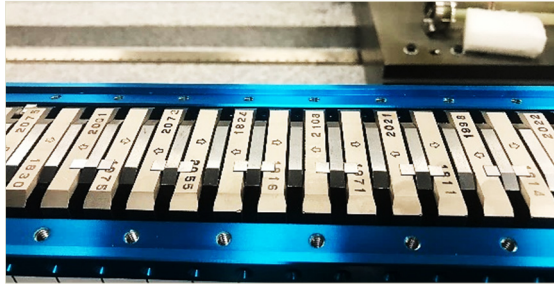
Figure 7: Photograph of twelve 0.2-mm-thick \times 5-mm-long surface shims placed on the bottom jaw with a 10-mm x-shift from the beam axis for the APS28#7 undulator.
