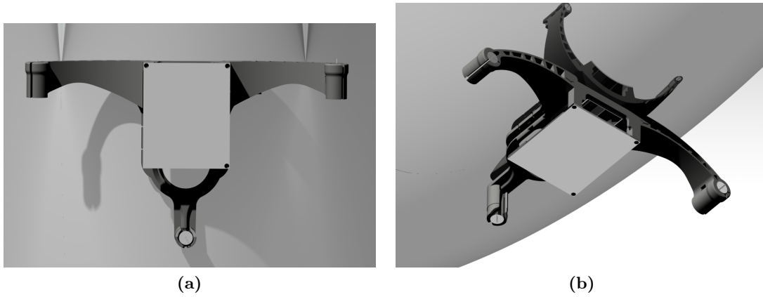
Figure 6.17: 3D rendering CAD model in CATIA of the Blimpduino system seen from the bottom with the control board (a) and from the front (b).
