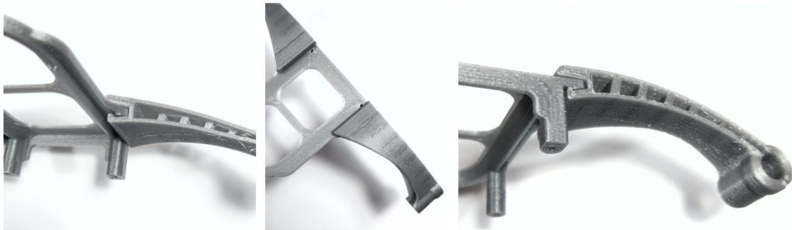
Figure 6.5: Fitting wings motors and frame of the Blimpduino 2. From [50].
