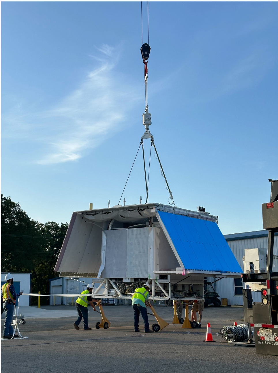
Figure 6: The GAPS scientific payload during the hang tests held at the Columbia Scientific Balloon Facility in Palestine.
