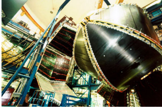
Figure 5.19: Photograph of the Region 3 drift chambers, with part of the time-of-flight detector in the background on the left [97].
