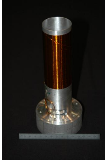
Figure 6.8: Photograph of the holding coil for longitudinal polarisation [128].
