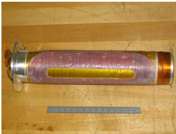
Figure 6.9: Photograph of the holding coil for transverse polarisation [128].
