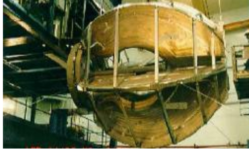
Figure 5.15: Photograph of the torus magnets before installation [97]. They are each 5 m long and 5 m in diameter.
