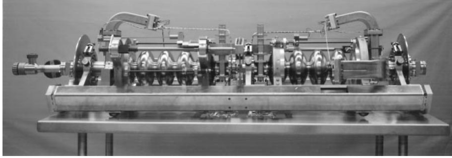
Figure 5.5: Photograph showing a typical CEBAF RF cavity pair or “cryounit” [86].
