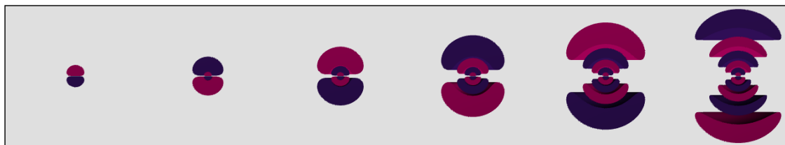
Figure 3.2: The 90-percentile plots of the p_z -orbitals in order from n = 2 to n = 6 in terms of the energy levels. The radius here has been stretched in the vertical axis so that the inner shells are made more obvious. The key thing to notice here is how the radial nodes increase with the energy level and occur very close to the nucleus of the atom. Remember also that these are only one of the possible three degenerate states for each energy level with l = 1 .
