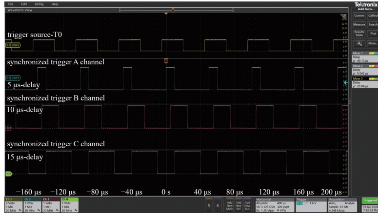
Fig. 10 Synchronized trigger signal test chart in internal trigger mode
