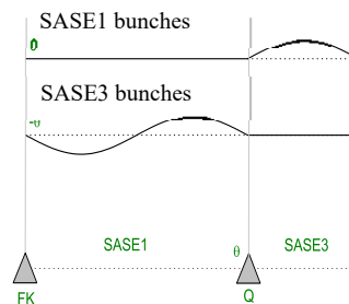
Figure 3: Betatron switcher used to suppress SASE3 bunches lasing in SASE1 and SASE1 bunches lasing in SASE3.
