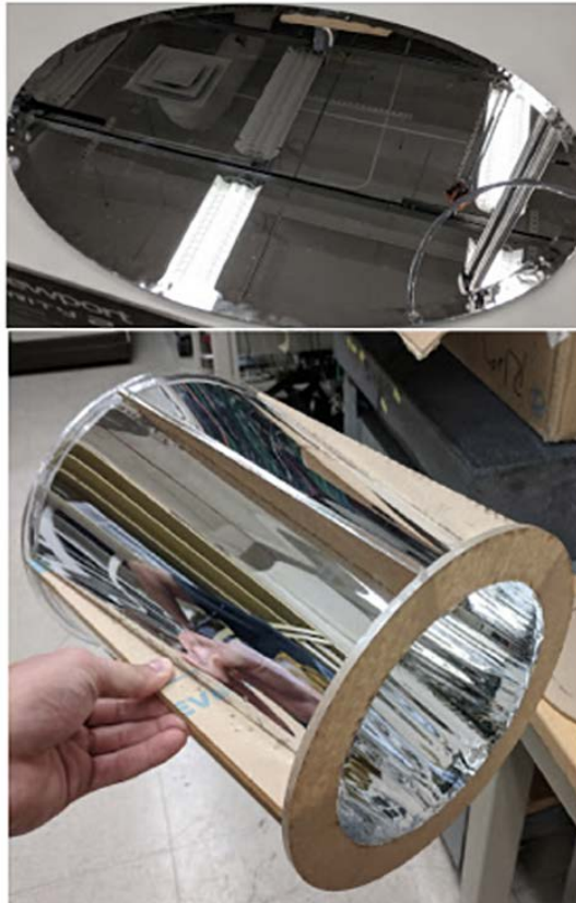
Figure C.14: Pictures of the finalized mirror and cone made out of spanned Mylar foil glued to the frame via stycast. The frames were laser cut and the irregularities on the foil were heat-shrank using a hair dryer.
