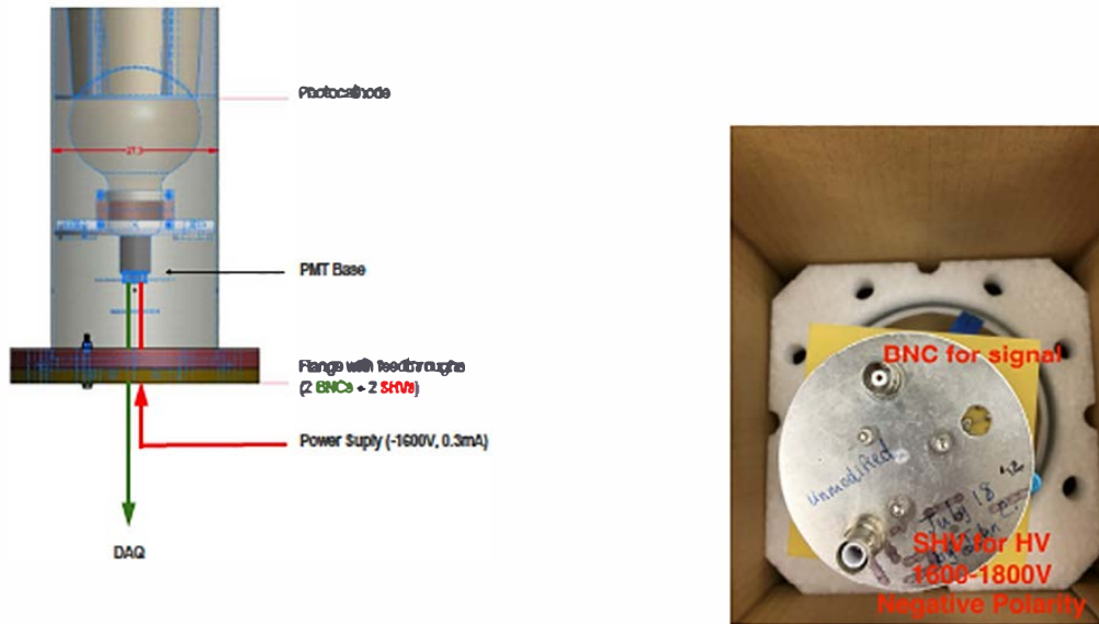
Figure C.19: Schematics and picture of electrical connections.
