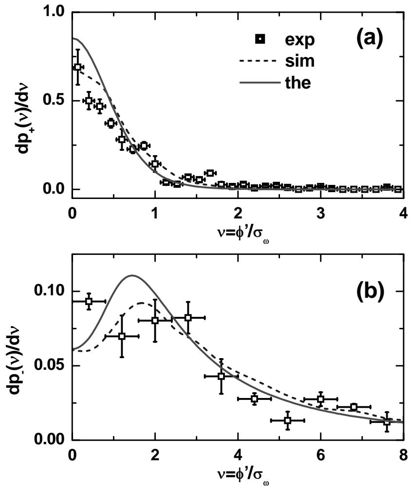
**Fig. 4** Distribution of phase derivative at the intensity maxima (a) and minima (b) normalized to the rms SASE FEL bandwidth. Experimental data (symbols), theoretical calculation (solid lines), and simulation results (dashed lines) are all presented. Note the different horizontal scales for (a) and the (b).
