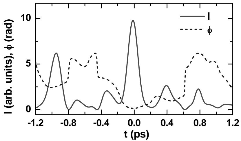
**Fig. 2** Field intensity (solid) and phase (dashed) as a function of time from a simulation with an electron bunch that is long compared to the coherence length using Eq. (1).
