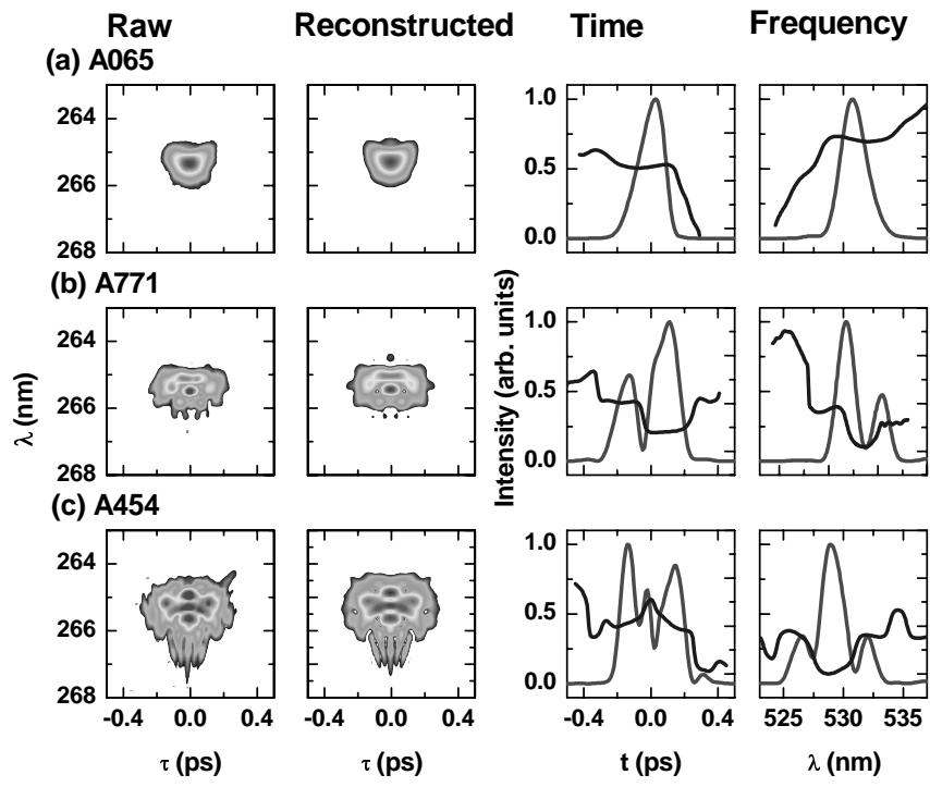
**Fig. 1 (a-c)** Examples of the raw and the reconstructed FROG traces, along with the field intensity and phase as a function of time and wavelength. Red: Intensity; Blue: Phase.
