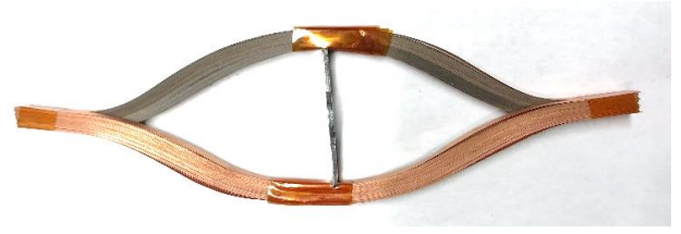
Fig. 4. Model of HTS coil assembled from 100 tape loops.
