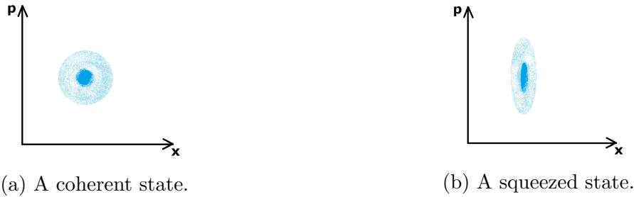
Figure 18: Two sketches comparing a coherent state to a squeezed state, as represented in phase space.
