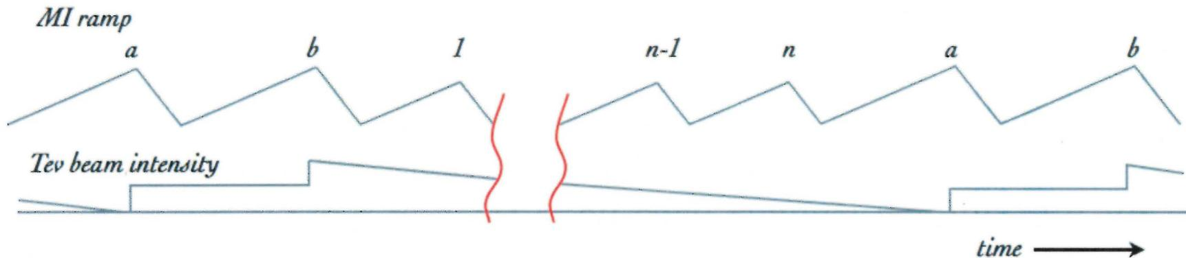
The Main Injector is being upgraded for the NO $\nu$ A program for which the 120-GeV cycle time will be  $T_n = 1.333$  s. To reach 150 GeV, the cycle time would be approximately  $T_k = 1.667$  s, assuming the maximum ramp rate of 240 GeV/s for NO $\nu$ A operation.
