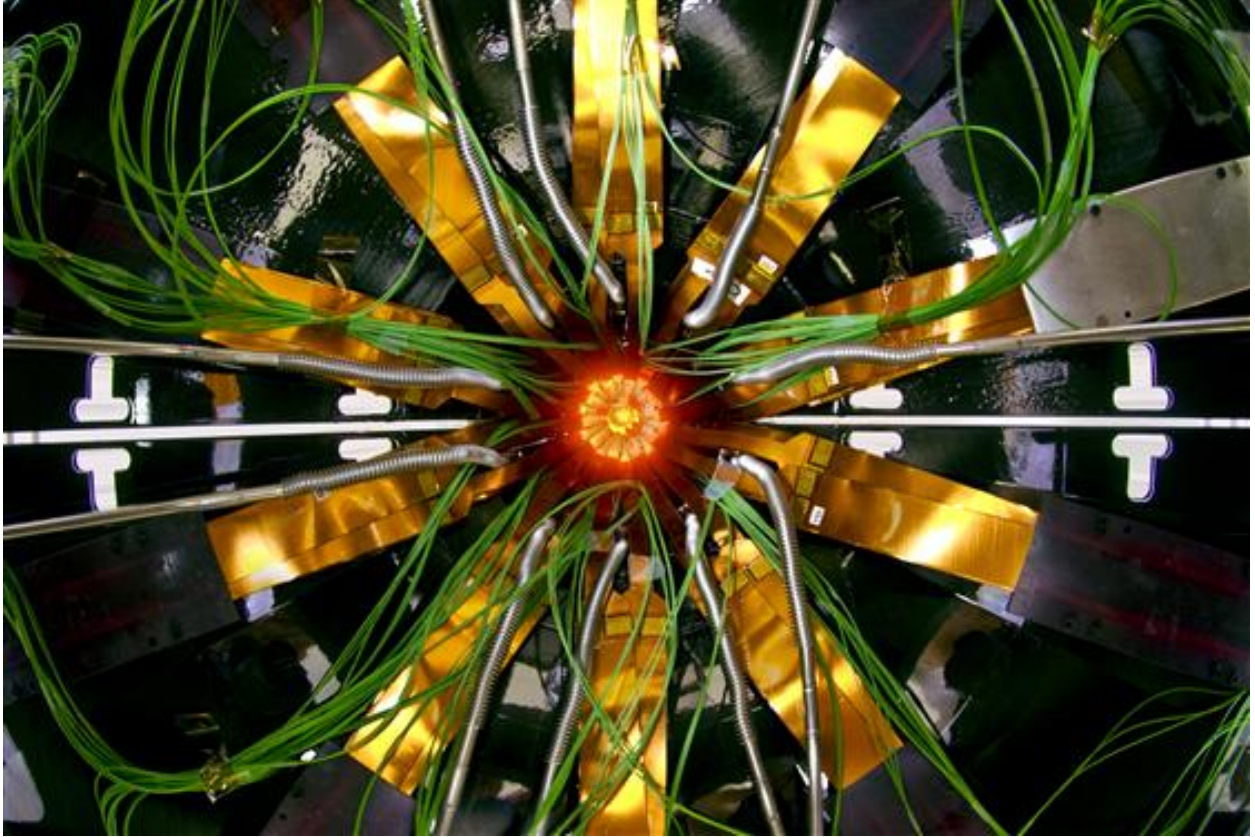
Figure 2.11: An SPD layer around the beam pipe. Image from ref [56].
