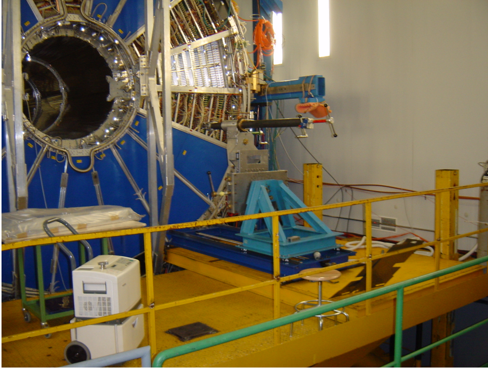
Figure 11.1: TPC with the Yellow Platform and the mounting tool.
