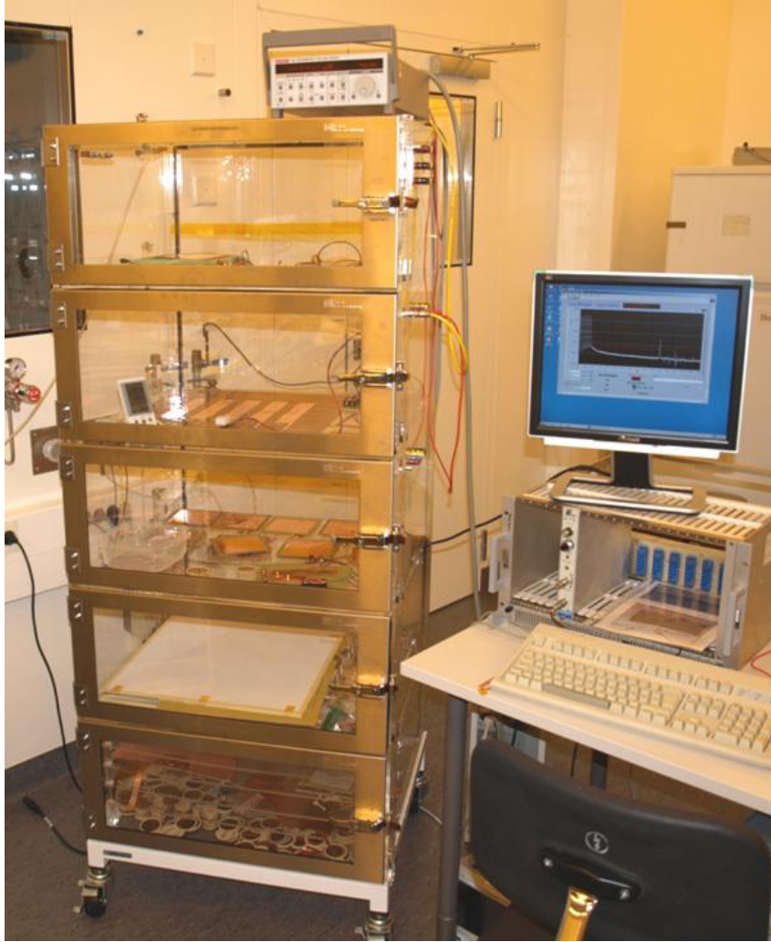
Figure 4.19: Leakage current measurement setup.
