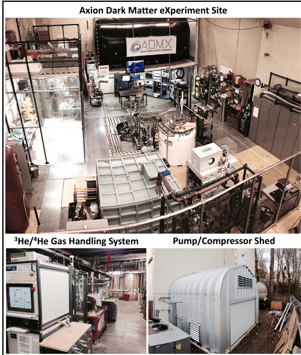
Figure 3.2: Images of the ADMX experimental site. The large superconducting magnet and experimental insert sit in a recess in the floor and are hidden from view in the center of the top of the figure. A ^4\text{He} recovery system cools the experiment, collects the blown off gas, re-compresses it in a pump shed (lower right hand side of the figure) and turns it back into a liquid to be used again. The lower left hand side of the figure shows a separate ^3\text{He}/^4\text{He} gas handling system used in conjunction with a dilution refrigerator.
