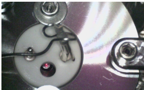
Figure 3: This shows the built-in alignment laser illuminating the back side of the cathode. The large white disk is the insulator in the AEI base that hold the cathode.
