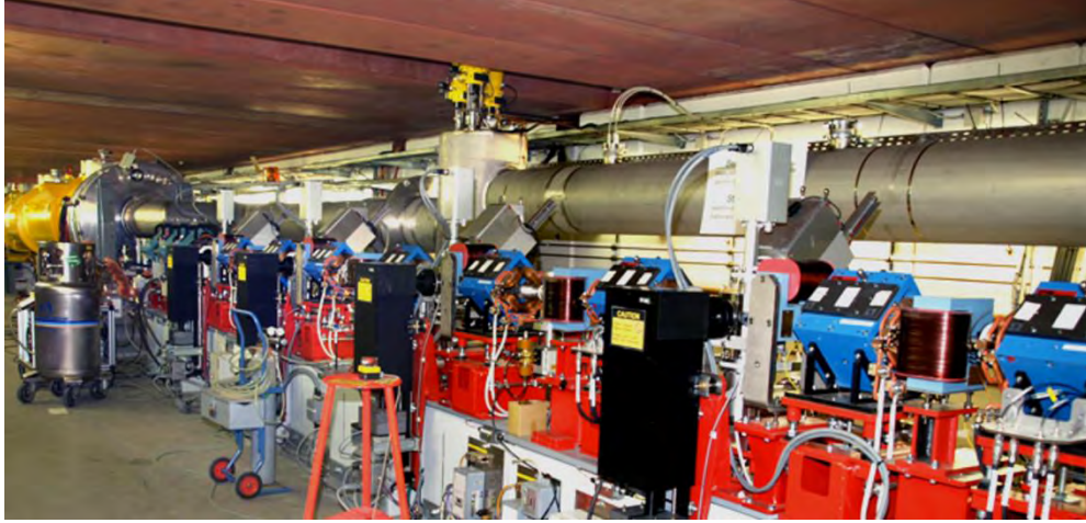
Figure 11.20. Picture of the diagnostic section of the FLASH injector. Four screen stations equipped with wire scanners in a FODO lattice with several quadrupole magnets are employed in measuring Twiss-parameters of the beam.
