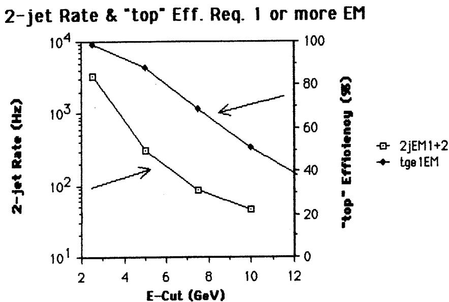
Note that if a cut is imposed to reduce the 2-jet rate to a few hundred, then the corresponding "top" efficiency drops to 60% or less.
