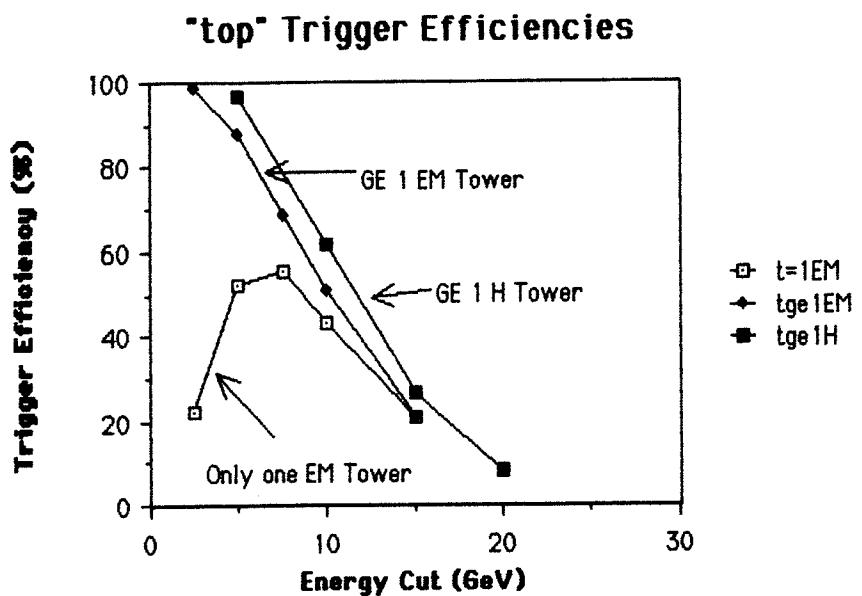
A plot of the "top" trigger efficiency along with the 2-jet rate requiring at least one EM tower to be above a cut, is included below.
