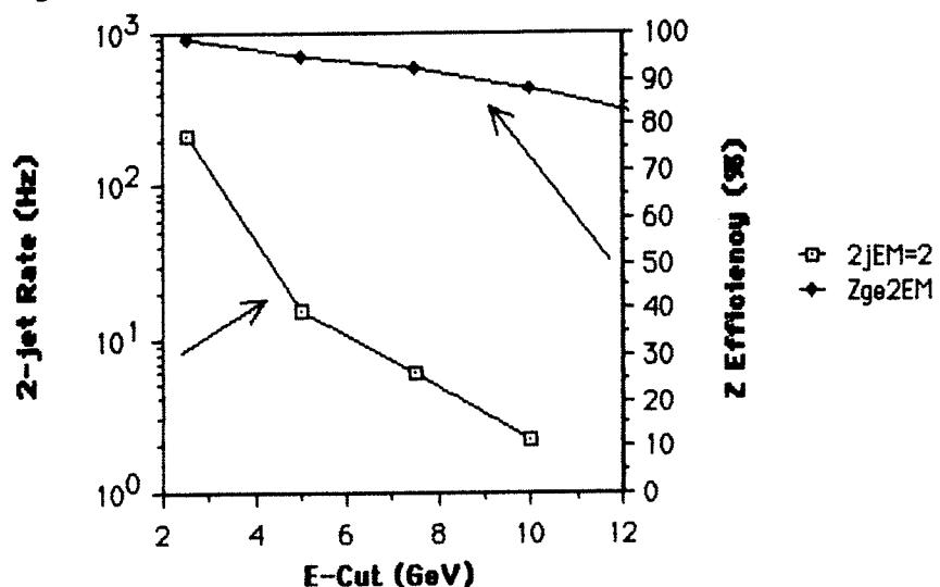
Requiring exactly two towers decreases the Z efficiency slightly but does not further decrease the 2-jet rate. This comparison is best seen in the following plot:
