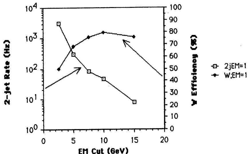
While the latter plot gives a somewhat lower 2-jet trigger rate for a given energy cut, it does so at the expense of the efficiency for the W. For example, at a cut of 10 GeV the efficiency is only 80% for the single tower trigger vs. nearly 90% for the trigger requiring one or more towers.
