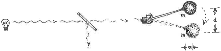
Fig.3 A photon impinges on a half-silvered mirror, so that only the transmitted part of its wave function is received by a device which if activated would move a macroscopic spherical lump of mass m and radius a through a distance d . Is there stage at which linear superposition between the two possible positions of the lump fails, and the lump actually becomes localized in one position or the other?
