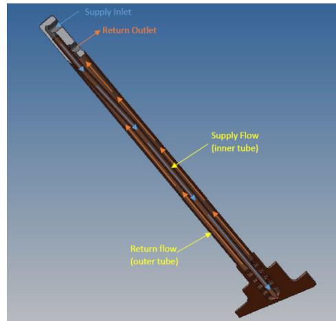
Figure 4: Illustration of the tube-in-tube configuration of PSH1. Cooling water enters from the inner tube and exits the outer tube passage.
