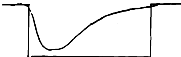
Figure 3.1a: The diagram of the relative timing between the ADC gate and the phototube pulses associated with the triggering interaction.
