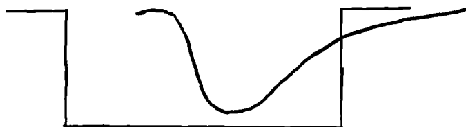
Figure 3.1b: The diagram of the relative timing between the ADC gate and the phototube pulses associated with the interaction occurring after the interaction that triggered the apparatus. The tail of the signal is not integrated.
