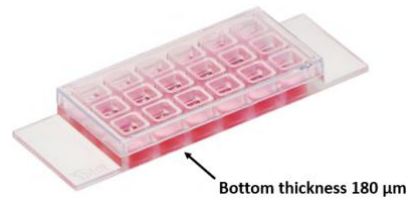
Figure 1. Holder used for the cells irradiations (6x3 well-plate array) [5]
