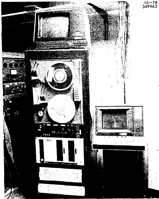
Fig. 2. One of the more elaborate ATROPOS systems consists of (from top to bottom): an Ann Arbor terminal (without keyboard) as an auxiliary display, a magnetic tape drive, an ECP, a dual floppy disk drive, the LSI-11 itself, and on the right, the Tektronix 4013 terminal which is used as the LSI-11 console and the graphics display device.
