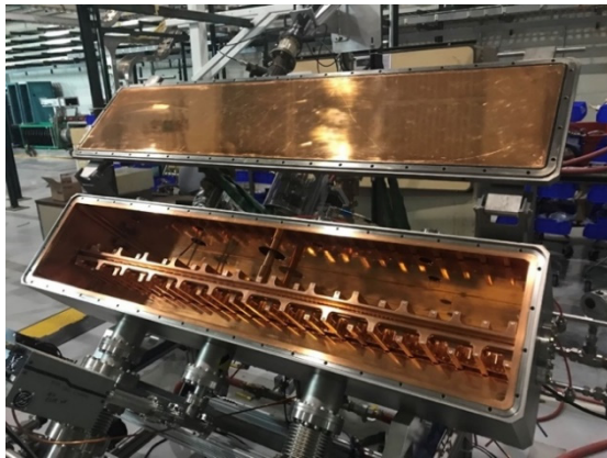
Figure 8: RFQ under test at the RFQ Test Stand.
