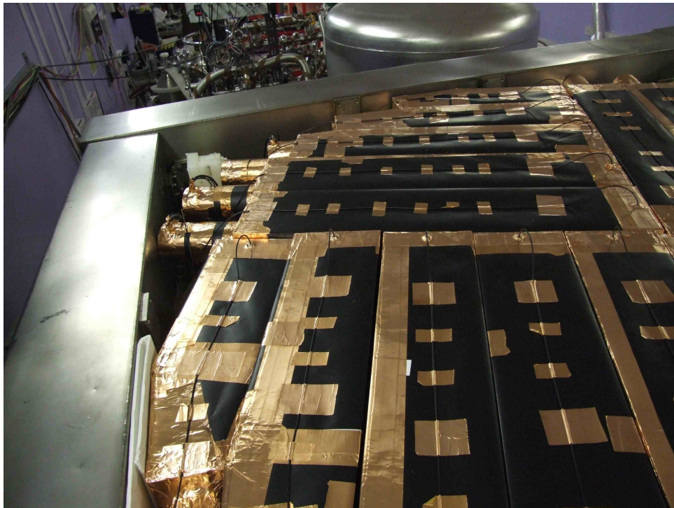
Figure 6.7: The lead castle built up to the level of the veto roof, the lead roof is built onto this leaving enough room for the LED fibre-optic cables which can be seen attached to the lower part of the roof scintillator slabs.
