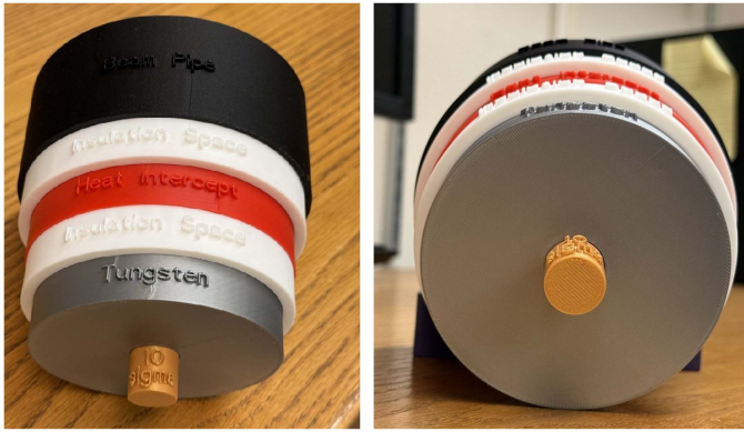
Fig. 3. 3D-printed radial build of the arc combined-function magnet. The main component in terms of size is the tungsten absorber (in silver).
