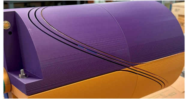
Fig. 9. Winding test on layer 3 of the CCT combined-function magnet.
