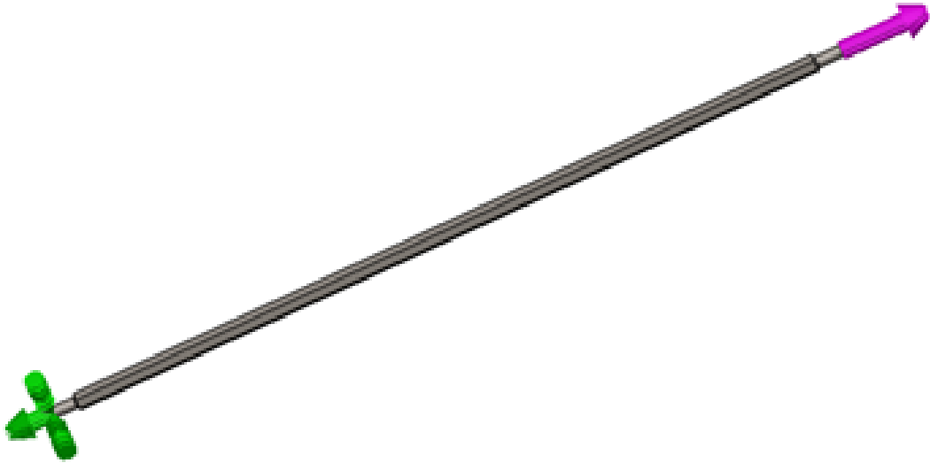
Figure A.20: Schematic of the FEA analysis of the rigid rods under tension.
