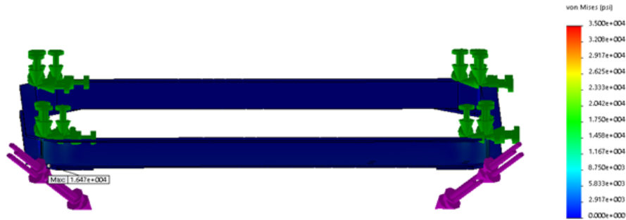
Figure A.47: FEA results for the aluminum components of the ballast attachment points with 5g applied at 45° towards the front, showing a maximum stress of 16.5 ksi.
