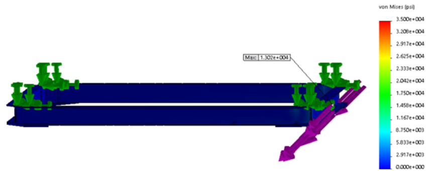
Figure A.44: FEA results for the aluminum components of the ballast attachment points with 5g applied at 45° to the right, showing a maximum stress of 13.0 ksi.
