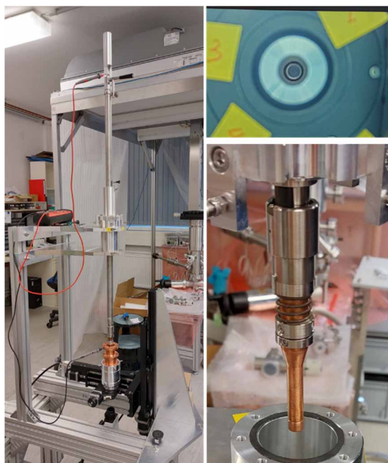
Figure 5: Test platform with a shortened version hand-rod and a cathode stalk.
