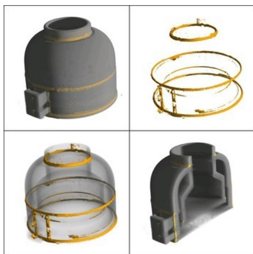
Fig. 2. Example image of assessment of soldering quality, semi-transparent 3D representation highlighting the Boron containing brazing solder distribution.
