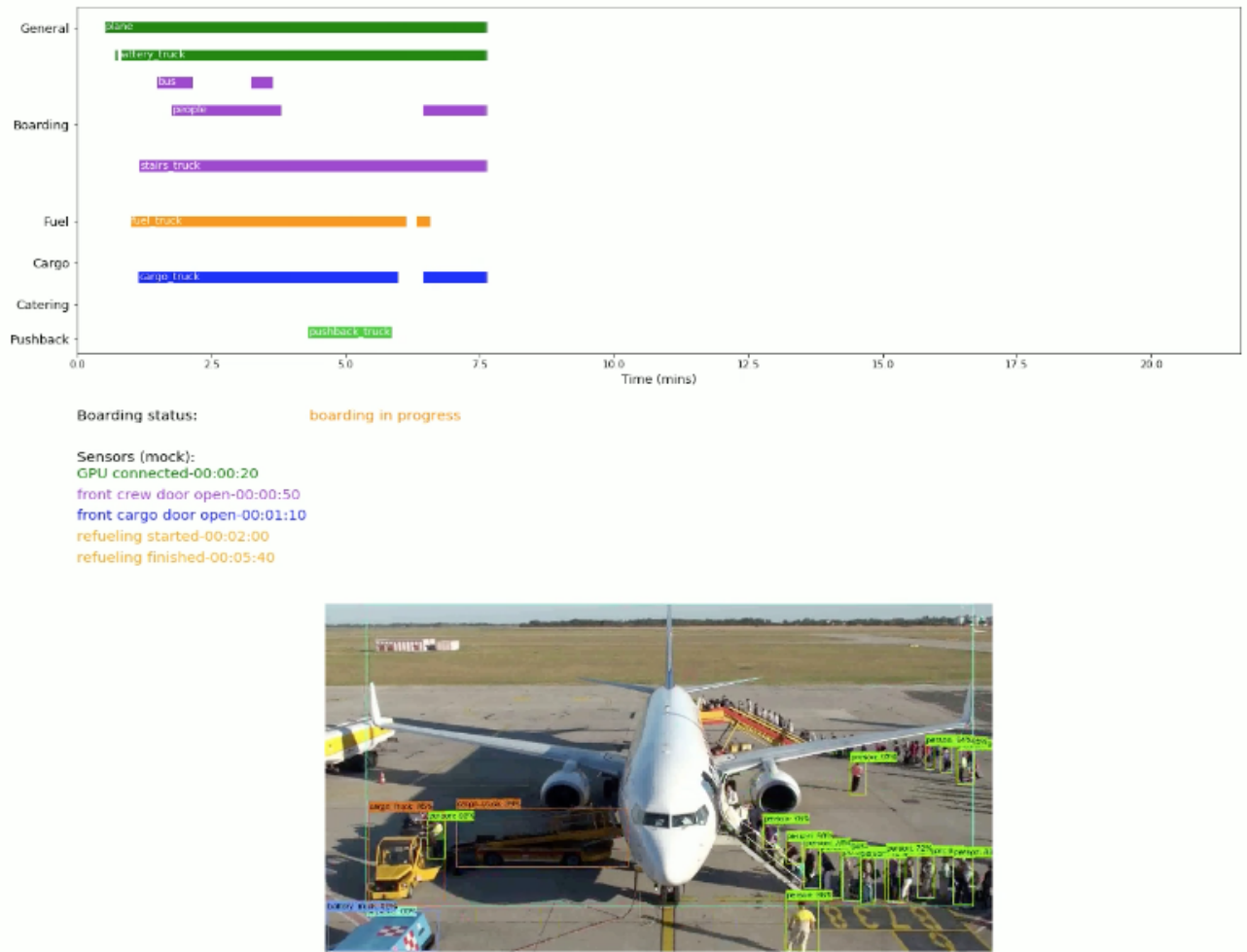
Figure B.6: Demonstration of how information from the object detection model and sensor data can feed into a display for turnaround monitoring.
