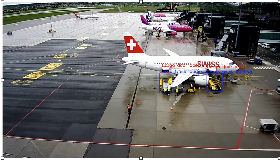
Figure B.4: Example output of our object detection model showing the cargo loading stage. The proximity of the cargo truck to an open cargo door flags it as loading.
