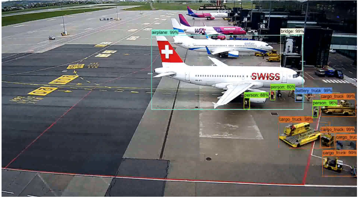
Figure B.3: Example output of our object detection model. Bounding boxes are displayed on the image as well as the class probability.
