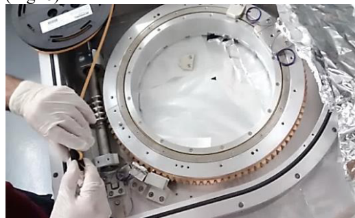
Figure 6: Vacuum cleaning procedures during assembly.
