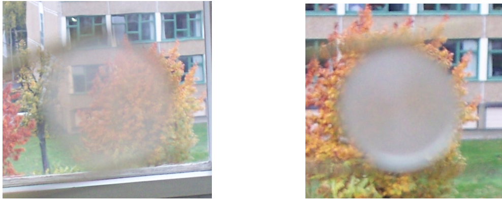
Figure 4.6: Acrylic sample 3 of Stock TUD before (left) and after the test (right). An increase of opacity is visible.
