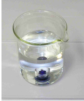
Figure 4.16: Inner container filled with ink in water.
