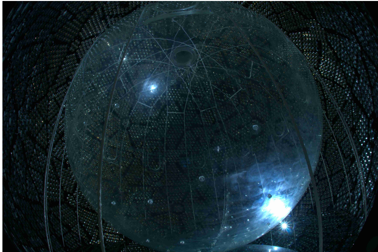
Figure 2.4: Picture of the SNO+ vessel from May 2014. The neck, the vessel, the hold down rope system and the PMTs are visible [Sin14].
