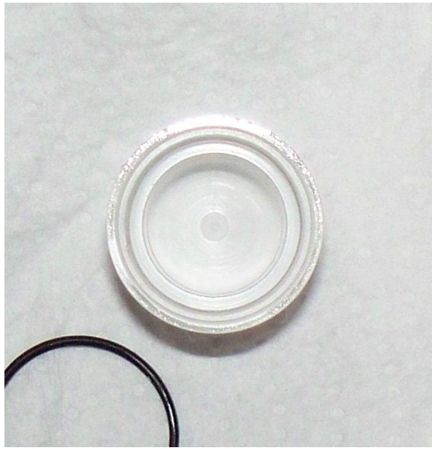
Figure 4.14: Outer container body after the pressure test. The O-ring edge is wet with LAB but all other parts are dry.
