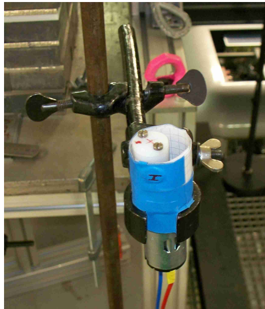
Figure 3.2: Titanium cylinder placed in a plastic holder before the activation. The number I marks the first niobium probe and below the motor is visible.
