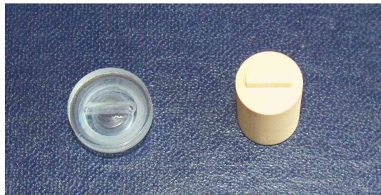
Figure 4.17: Inner container lid with slit (left) and plastic rod used for screwing it (right).
