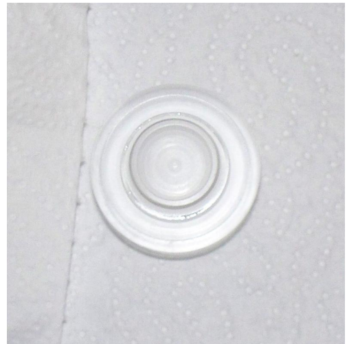
Figure 4.15: Outer container lid after the pressure test. The O-ring edge is wet with LAB but all other parts are dry.
