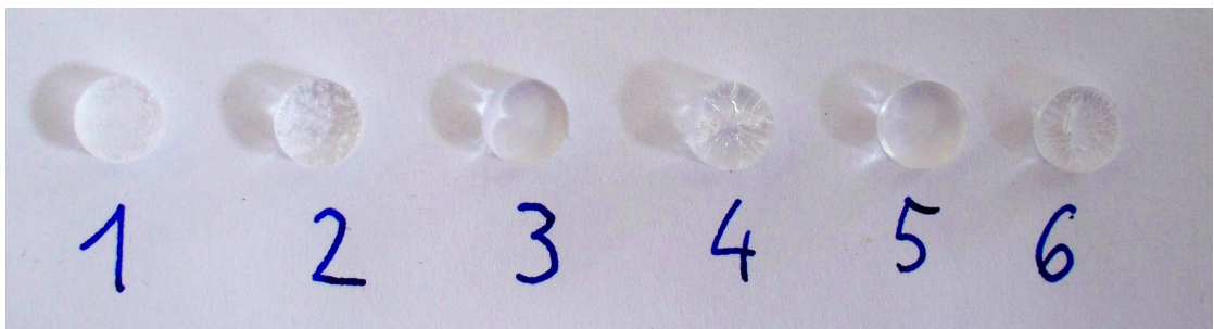
Figure 4.5: Broken samples after the first ethanol test.
