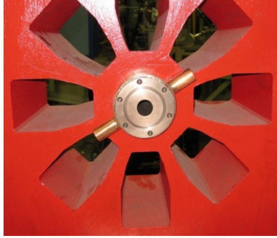
Figure 3.8: Picture of the tungsten plug in the central aperture of the collimator closest to the target. Acceptance holes are also visible.
