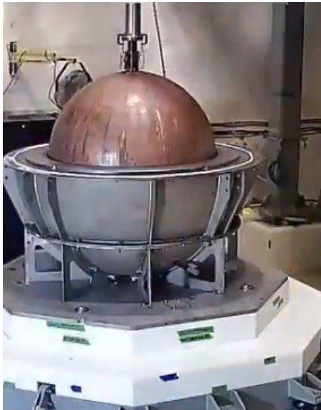
Figure 3.10: NEWS-G at SNOLAB. Left picture shows the installation of the detector inside of its let shielding. The right illustration shows the detector and the different layers of shielding, courtesy of K. Dering.
